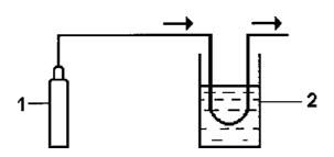
1 Purging gas (no. 2 in Figure C.3) 2 Cooling trap with liquid nitrogen (no. 7 in Figure C.3)
