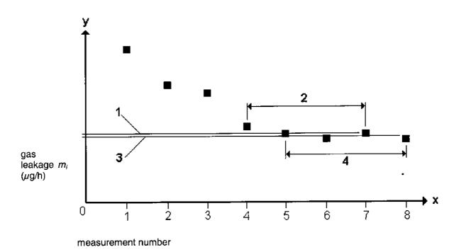
1 Mean value of measurements 4 to 7; standard deviation less than 0,25  $\mu$ g/h
