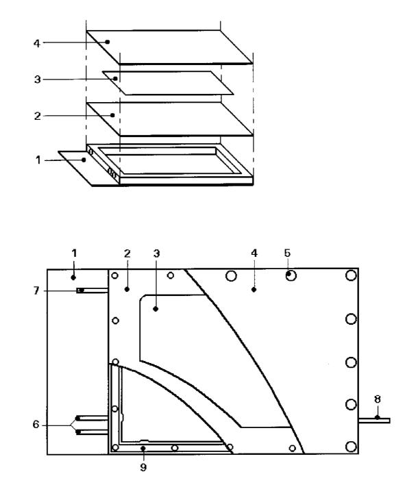
1 Lower part6 Purging gas in and out2 Metal foil7 Protective gas in3 Mat8 Protective gas out4 Cover9 Annular groove
