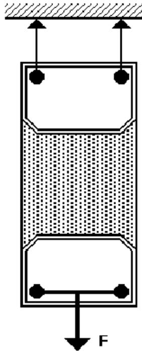
**Figure F.1 - Example of the principle of the adhesion test.**
