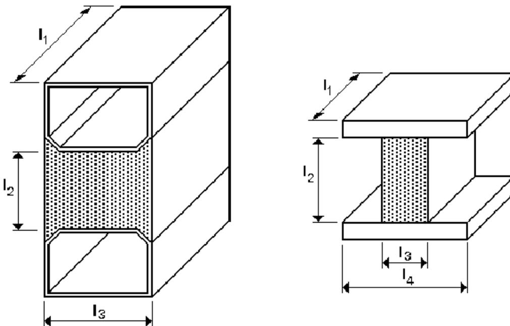
Spacer-spacer sample:  $l_1 = 20$  mm,  $l_2 \geq 11,5$  mm and  $l_3 =$  spacer width
