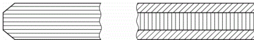
Figure 14 — Smooth ground edge (no blank spots)
