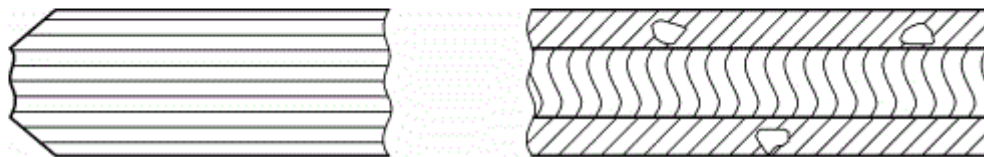
Figure 12 — Arrissed edge (with blank spots)
