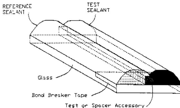
FIG. 3 View of Test Specimen
