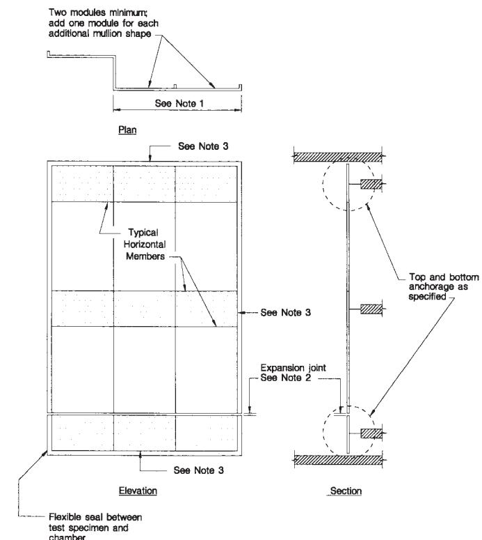
NOTE 1—Width of typical specimen if no corners are included in system or project.
