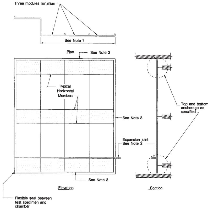
NOTE 1—Width of typical specimen if no comers are included in system or project.
