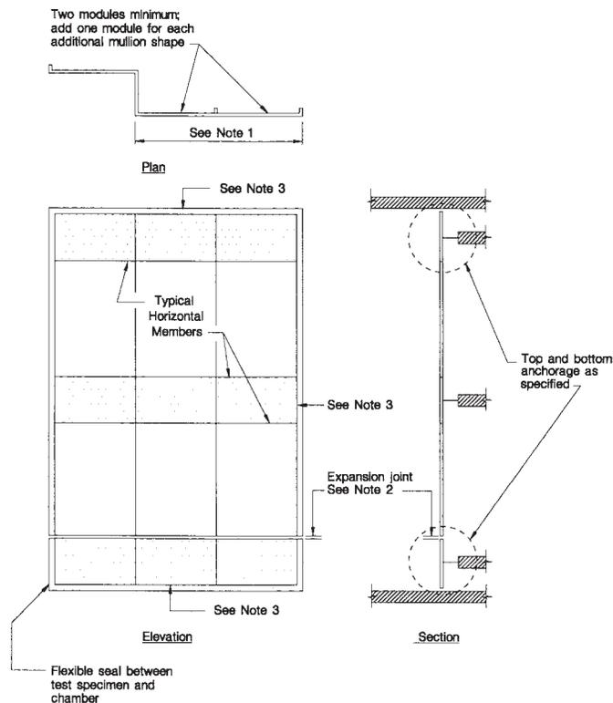
NOTE 1—Width of typical specimen if no comers are included in system or project.
