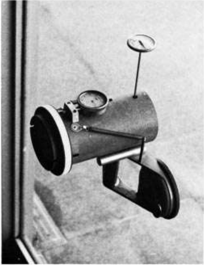
FIG. 4 Vertical Attachment Fixture and Frost-Point Apparatus in Use
